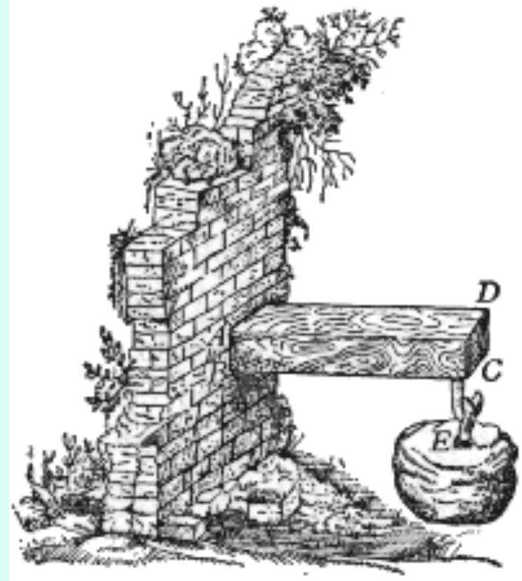
*Galileo's illustration of bending test, "Two New Sciences"*
