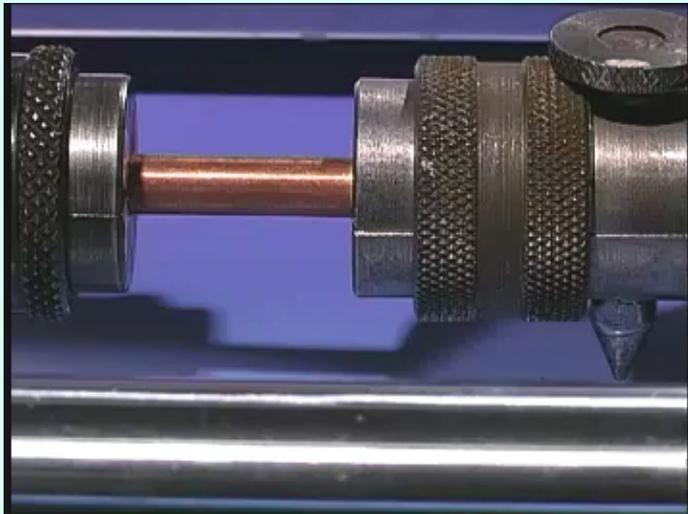
Ductile fracture of annealed copper, Courtesy of DoITPoMS, The University of Cambridge
