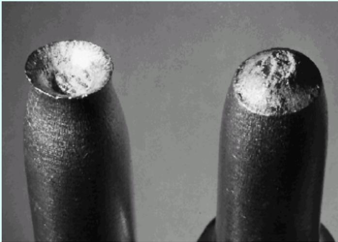
Cup-and-cone fracture in Al
